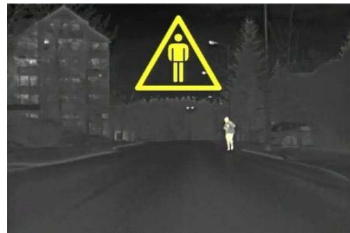
Figure 2. BMW Night-vision Camera Detection System
